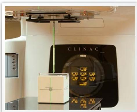
**User's Guide Includes:** An enhanced Lehmann Yoke testing procedure for confirmation of the source to surface distance (SSD).
